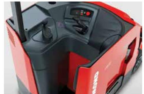
The ergonomically designed compartment and single, low-force deadman pedal reduce operator fatigue and enhance comfort.
